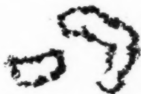
10 shots at 100 yards rest, .25-caliber Roberts rifle, 8X Fecker scope. F. A. No. 70 primer, 18.5 grs. No. 4227, 117-gr. Western boat-tail open-point bullet. Shot by Manley A. Butts, Sept. 26, 1936
